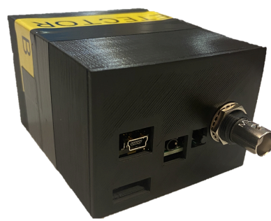
Figure 3: (A) and (B) shows the front and the back of the detector respectively. As seen, the OLED screen, LED, microSD Card Slot, BNC receptacle, reset button, micro USB slot, and the coincidence connection are aligned with the grooves made in the plastic casing.
