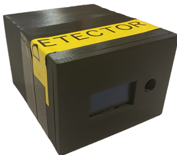
Figure 3: (A) and (B) shows the front and the back of the detector respectively. As seen, the OLED screen, LED, microSD Card Slot, BNC receptacle, reset button, micro USB slot, and the coincidence connection are aligned with the grooves made in the plastic casing.
